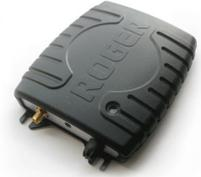
A single ROGER-GPS Repeater Package is enough to provide a GPS L1 (1.57542 GHz), Glonass G1 (1.602 GHz), and Galileo E1 (1.57542 GHz) indoor signal coverage area of ~ 10,700 ft<sup>2</sup> and a distance of up to 164 ft. from the repeater center. Mount the external antenna on the roof of the building and connect the cable supplied with the kit to the antenna and to the repeater installed indoors.
