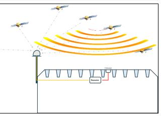
tracking of GNSS signals when moving from indoors out.
