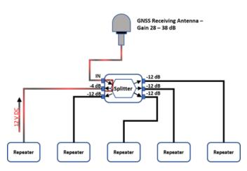
DC power is passed from the chaining output to the input connector for a line amplifier and/or to the GNSS receiving antenna. The ROGER™-GNSS Splitter is a one to five signal splitter with one port with an output of -4 dB (DC passthrough) and four ports with an output of -12 dB. The splitter is easy to use and permits a wide range of system configurations.
